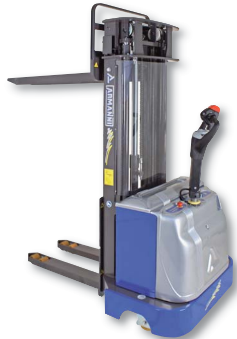
Delta TRX FL AC 145/40E Triplex Freihubmast, FL = Free Lift
